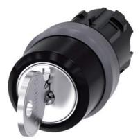
RONIS key-operated switch, 22 mm, round, plastic with metal front ring, lock number SB30, with 2 keys, 3 switch positions I>O<II, momentary contact on the left, latching on the right, actuating angle 2x45°, 10:30h/12h/13:30h, Key removal O+II, possible special locks: SB31, 421, 455, Z=50-unit packaging
