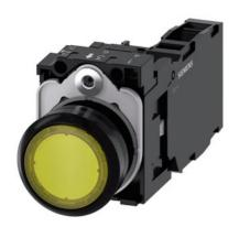
Illuminated pushbutton, 22 mm, round, plastic, yellow, pushbutton, flat, momentary contact type, with holder, 1 NO+1 NC, LED module with integrated LED 110 V AC, screw terminal, with laser labeling, upper case and lower case, always upper case at beginning of line
