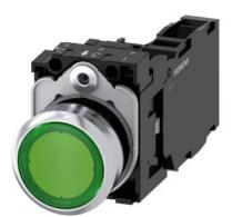
Illuminated pushbutton, 22 mm, round, metal, shiny, green, pushbutton, flat, momentary contact type, with holder, 1 NO+1 NC, LED module with integrated LED 110 V AC, screw terminal, with laser labeling, inscription or symbol Customer-specific selection with SIRIUS ACT configurator (CIN)
