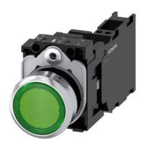
Illuminated pushbutton, 22 mm, round, metal, shiny, green, pushbutton, flat, momentary contact type, with holder, 1 NO+1 NC, LED module with integrated LED 230 V AC, spring-type terminal, Z=20-unit packaging
