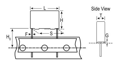
General Information Series F871 Dielectric Metallized Polypropylene Style Radial Features MKP EMI Safety RoHS Lead Wire Leads Safety Class X1 Qualifications ENEC, UL, cUL, CQC AEC-Q200 No THB Performance No Component Weight 2.037 g Miscellaneous ClimCat: 40/110/56/C. Shelf Life 104 Weeks
