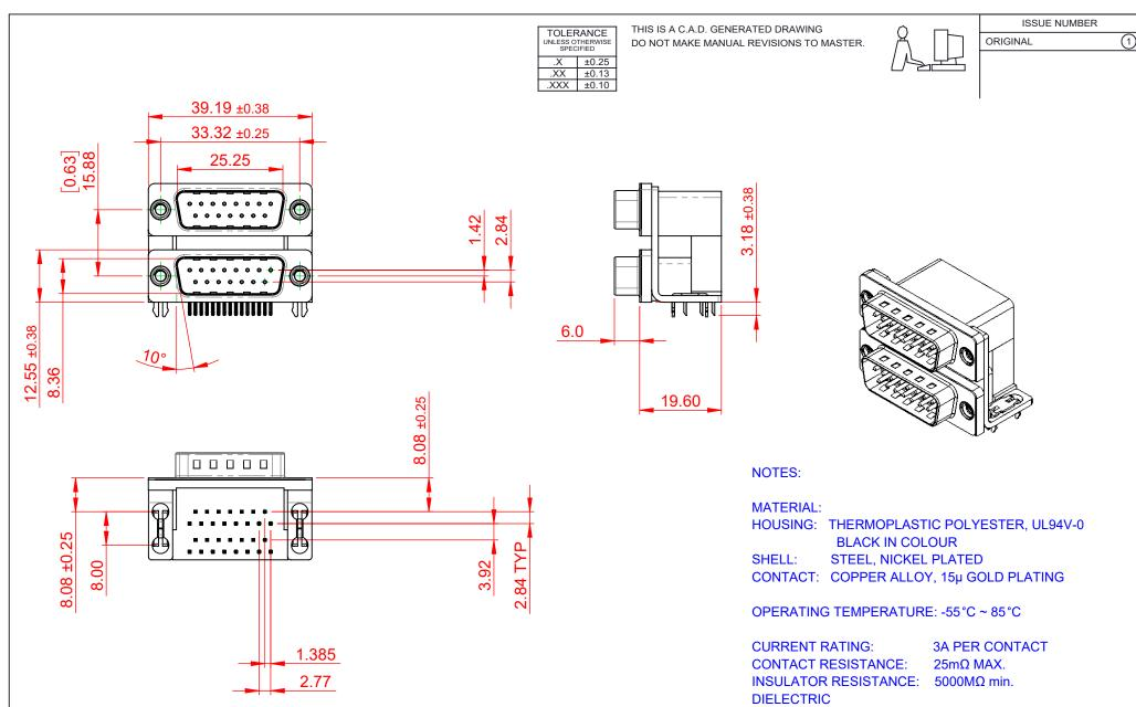
WITHSTANDING VOLTAGE: 1000V AC rms
