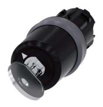
Key-operated switch BKS, 22 mm, round, plastic with metal front ring, special lock, with 2 keys, 2 switch positions O-I, latching, actuating angle 90°, 10:30h/13:30h, key removal O, Note: BKS locking systems E1 - E25 supplied without key
