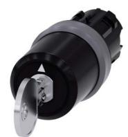
Key-operated switch BKS, 22 mm, round, plastic with metal front ring, lock number S1, with 2 keys, 3 switch positions I>O<II, momentary contact on the left, latching on the right, actuating angle  $2x45^{\circ}$ , 10:30h/12h/13:30h, key removal O, with laser labeling, upper case and lower case,
