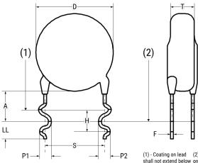
(1) - Coating on lead (2) - Point of support shall not extend below on printed cardboard. this line.
