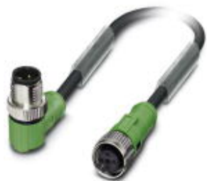
Sensor/actuator cable, 3-position, Variable cable type, Plug angled M12 SPEEDCON, A-coded, on Socket straight M12 SPEEDCON, A-coded, cable length: Free input (0.2 ... 40.0 m)
