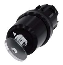
key-operated switch Siemens, 22 mm, round, plastic, lock number SSG10, with 2 keys, 2 switch positions O<I, momentary contact type, actuating angle 45°, 10:30h/12h, key removal O Z=50-unit packaging
