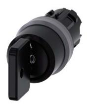
Key-operated switch O.M.R, 22 mm, round, plastic with metal front ring, lock number 73034, black, with 2 keys, 3 switch positions I-O<II, left latching, right momentary contact type, actuating angle 2x45°, 10:30h/12h/13:30h, key removal I, with laser labeling, upper case and lower case, always upper case at beginning of line
