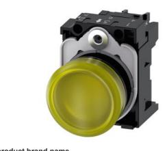
Indicator lights, 22 mm, round, plastic, yellow, lens, smooth, with holder, LED module, with integrated LED 24 V AC/DC, screw terminal, with laser labeling, symbol number according to, ISO 7000 or IEC 60417
