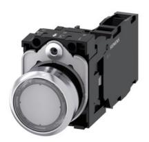
Illuminated pushbutton, 22 mm, round, metal, shiny, clear, pushbutton, flat, momentary contact type, with holder, 1 NO+1 NC, LED module with integrated LED 24 V AC/DC, screw terminal, with laser labeling, upper case
