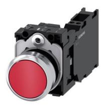
Pushbutton, 22 mm, round, metal, shiny, red, pushbutton, flat, momentary contact type, with holder, 1 NO+1 NC, spring-type terminal, with laser labeling, upper case and lower case, always upper case at beginning of line
