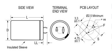
General Information Series ALC80 Dielectric Aluminum Electrolytic Description Snap-In, Aluminum Electrolytic RoHS Lead 3 Pin Short AEC-Q200 No Halogen Free Yes Component Weight 165 g Notes Dimensions D And L Include Sleeving. Shelf Life 156 Weeks
