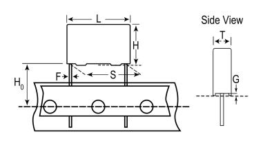
General Information Series Dielectric Metallized Polypropylene Style Radial Features MKP EMI Safety RoHS Yes Lead Wire Leads Safety Class X1 Qualifications ENEC, UL, cUL, CQC AEC-Q200 No THB Performance No Component Weight 5.959 g Miscellaneous ClimCat: 40/110/56/B Shelf Life 104 Weeks
