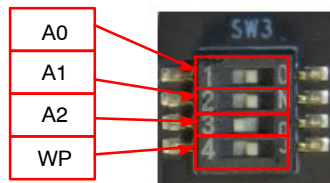
Figure 8. Address Switch Locations in their Default Positions. The First Switch (ADR0) and the Second Switch (ADR1) of SW3 are Set to ON
