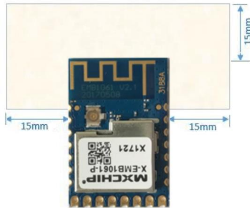
Figure 2.2 Minimum PCB Clearance Area
