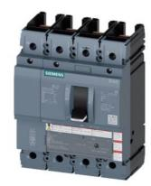
circuit breaker 3VA5 UL frame 250 breaking capacity class C 100kA @ 480V 4-pole, line protection TM210, FTFM, In=110A overload protection Ir=110A fixed short-circuit protection Ii=10 x In N conductor protection 100% without connection
