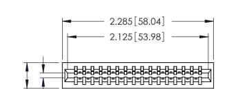
Card Slot Accepts .054 (1.37) to .070 (1.78) Thick P.C. Board
