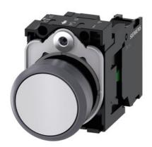
Pushbutton, 22 mm, round, plastic with metal front ring, white, pushbutton, flat, momentary contact type, with holder, 1 NO, screw terminal, with laser labeling, upper case and lower case, always upper case at beginning of line
