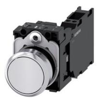
Pushbutton, 22 mm, round, metal, shiny, white, pushbutton, flat, momentary contact type, with holder, 1 NO+1 NC, spring-type terminal, with laser labeling, symbol number according to, ISO 7000 or IEC 60417
