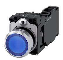
Illuminated pushbutton, 22 mm, round, metal, shiny, blue, pushbutton, flat, momentary contact type, with holder, 1 NO+1 NC, LED module with integrated LED 24 V AC/DC, screw terminal, with laser labeling, upper case and lower case, always upper case at beginning of line
