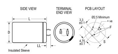
General Information Series ALC70 Dielectric Aluminum Electrolytic Description Snap-In, Aluminum Electrolytic RoHS Lead 3 Pin Short AEC-Q200 No Halogen Free Yes 40 g Component Weight Notes Dimensions D And L Include Sleeving. Shelf Life 156 Weeks
