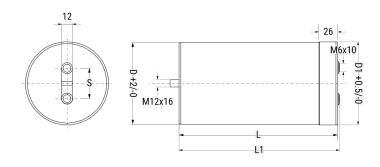
General Information Series C44U-M Dielectric Metallized Polypropylene Style DC Filtering, Energy Storage Features RoHS With Exemptions **REACH** SVHC (Pb - CAS 7439-92-1) SCIP Number cc1c1ec4-db9e-4815-b26b-e8a34ddfb776 Screw Terminals M6 Lead AEC-Q200 Nο Component 1840 g Weight Thermal Resistance = 2.6 C/W. Weight = 9200 Miscellaneous grams.
