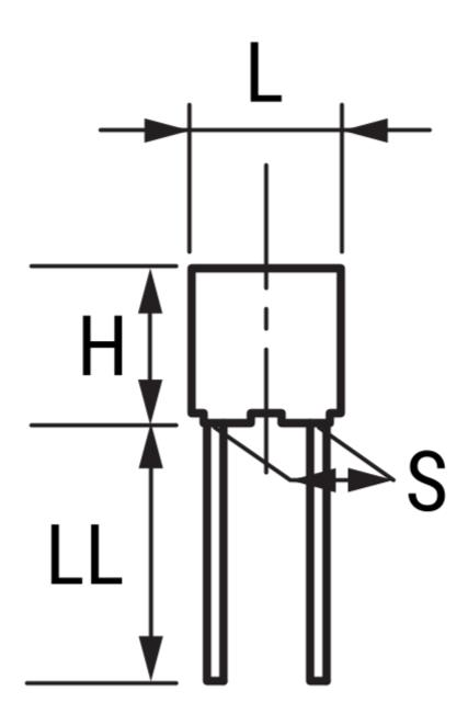
Click <u>here</u> for the 3D model. **Dimensions** L 7.2mm +0.3mm
