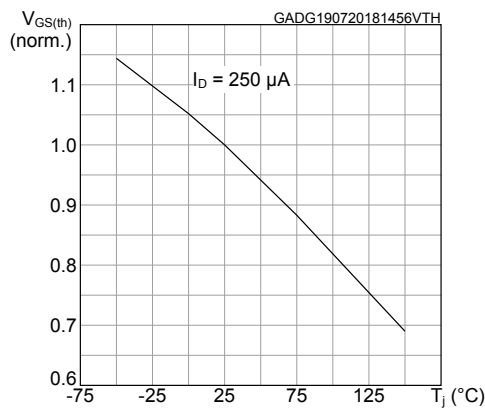
Figure 9. Normalized gate threshold voltage vs temperature
