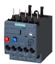
Overload relay 7.0...10 A Thermal For motor protection Size S00, Class 10 Contactor mounting Main circuit: Screw Auxiliary circuit: Screw Manual-Automatic-Reset
