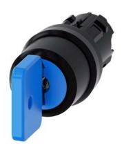
Key-operated switch O.M.R, 22 mm, round, plastic, lock number 73038, blue, with 2 keys, 3 switch positions I-O-II, latching, actuating angle 2x45°, 10:30h/12h/13:30h, Key removal I+O+II, with laser labeling, upper case
