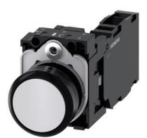
Pushbutton, 22 mm, round, plastic, white, pushbutton, flat, momentary contact type, with holder 1 NO+1 NC, screw terminal, with laser labeling, upper case and lower case, always upper case at the beginning of the word
