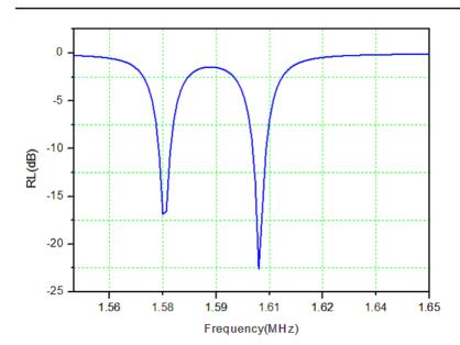
Return Loss characteristic shows a dual band response for GPS/Galileo & GLONASS R.H.).
