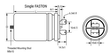
General Information Series C87 Dielectric Film/Foil Polypropylene Style Aluminum Case, Plastic Cover, Spun Seal Description Features Spun Seal, Safety Class S2, UL\_94 V0 Disk RoHS Yes Lead Fast On (1+1) UL, VDE, CQC, CSA (600VAC), UL\_94 V0 Qualifications Disk AEC-Q200 No Component 58 g Weight
