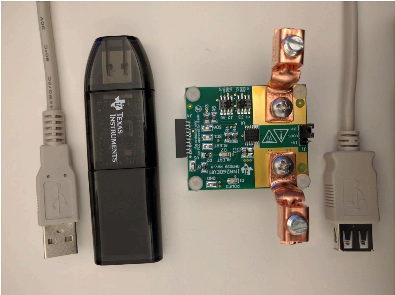
Figure 1-1. Hardware Included with the INA260EVM Kit
