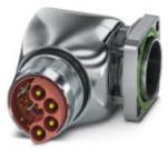
Device connector for front wall, angled rotatable, for standard and SPEEDCON interlock, M23, No. of pos.: 8+4+PE, type of contact: Pin, Crimp connection, Axial O-ring, 4x Ø 3.2, flange dimensions: 28 mm x 28 mm
