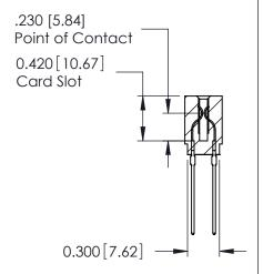
725 Series Ultra-Mate Card Edge Connector - Press Fit Part Number: 725-048-541-201 **EDAC INC** THESE DRAWINGS AND SPECIFICATIONS
