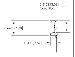
ACAD REFERENCE NO. 737 Series Ultra-Mate Card Edge Connector - Press Fit DRAWN: Part Number: 737-012-541-101 CHECKED: **EDAC INC** SCALE: THESE DRAWINGS AND SPECIFICATIONS ARE THE PROPERTY OF EDAC INC.,AND TORONTO, ONTARIO SHALL NOT BE REPRODUCED, OR COPIED DRAWING NUMBER CANADA OR USED AS THE BASIS FOR THE 737-ENG MASTER MANUFACTURE OR SALE OF APPARATUS YOUR CONNECTION TO QUALITY & SERVICE WITHOUT WRITTEN PERMISSION.
