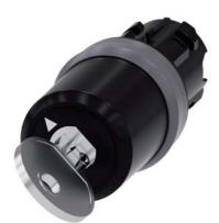
key-operated switch Siemens, 22 mm, round, plastic with metal front ring, lock no. LSG1, with 2 keys, 2 switch positions O-I, latching, actuating angle 90°, 10:30h/13:30h, key removal O+I, with laser labeling, upper case and lower case, always upper case at beginning of line
