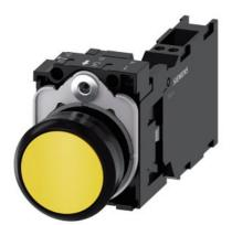
Pushbutton, 22 mm, round, plastic, yellow, pushbutton, flat, momentary contact type, with holder 1 NO+1 NC, spring-type terminal, with laser labeling, upper case and lower case, always upper case at the beginning of the word
