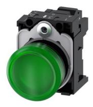
Indicator lights, 22 mm, round, plastic, green, lens, smooth, with holder, LED module, with integrated LED 110 V AC, spring-type terminal, with laser labeling, upper case and lower case, always upper case at the beginning of the word
