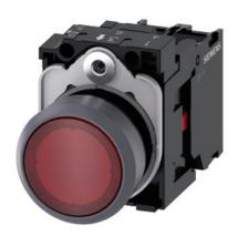
Illuminated pushbutton, 22 mm, round, plastic with metal front ring, red, pushbutton, flat, momentary contact type, with holder, 1NC, LED module with integrated LED 230 V AC, screw terminal, with laser labeling, upper case and lower case, Always upper case at the beginning of the word
