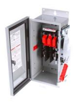
Siemens Low Voltage Circuit Protection Heavy Duty Safety Switches. Type: ENCLOSED, SAFETY SWITCH Std: UL V. Rating: 240V A. Rating: 30 A Wattage: 2W No. Of Poles: 2P F. Rating: 60Hz Action: SINGLE THROW Material: 304SS Enclosure: TYPE 12. 2-3 point mounting holes. Insulation: YES O. Cycles: 10000 O. Temperature: (-20F-120F) AMBIENT TEMPERATURE Environmental Conditions: INDUSTRIAL
