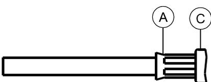
Slide ferrule A over braid and crimp to connector body C as close as possible.
