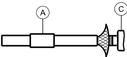
Splay out braid and insert cable in connector body C.
