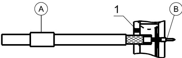
Push contact B over inner conductor of cable to about cable-dielectric and crimp with cavity 1.
