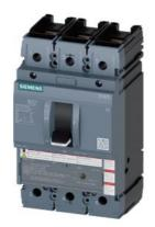
circuit breaker 3VA5 UL frame 250 breaking capacity class C 100kA @ 480 V 3-pole, line protection TM230, FTAM, In=200A overload protection Ir=200A fixed short-circuit protection li=5...10 x In UL489 SB (naval), 50 deg. cel. nut keeper kit on both sides
