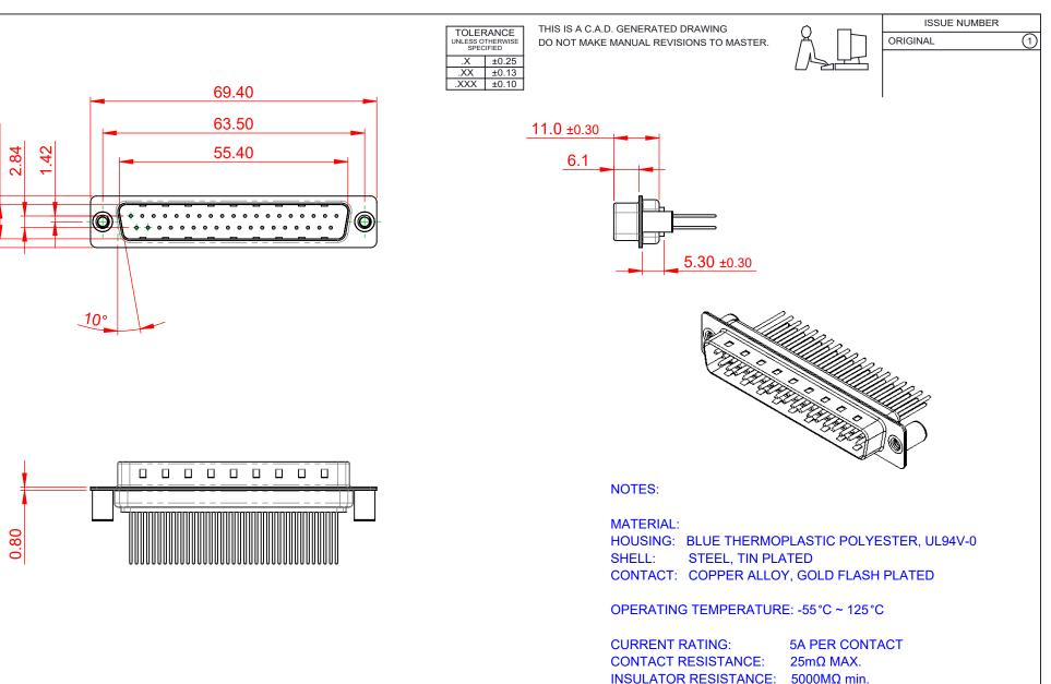
DIELECTRIC WITHSTANDING VOLTAGE: 1000V AC rms
