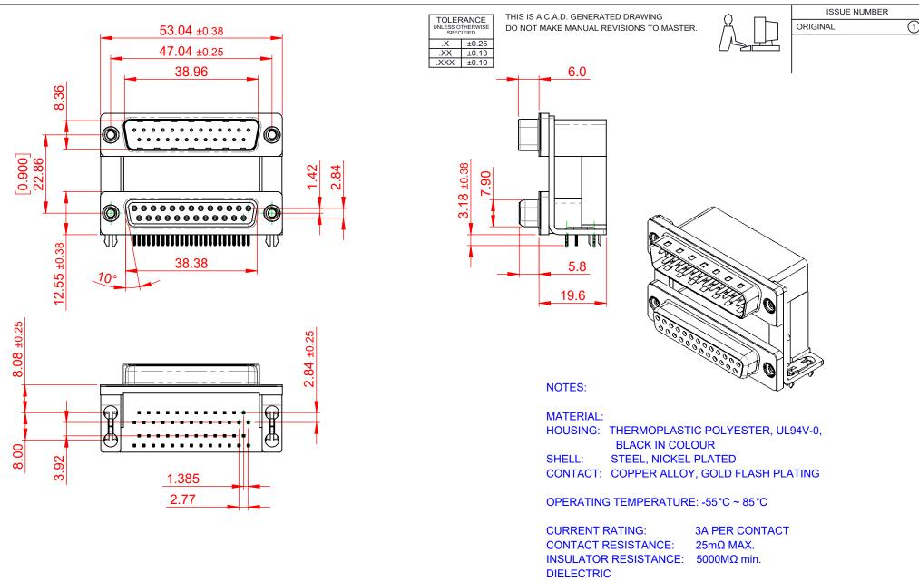
WITHSTANDING VOLTAGE: 1000V AC rms
