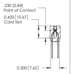
ACAD REFERENCE NO. 725-ENG MASTER 725 Series Ultra-Mate Card Edge Connector - Press Fit SEGAHOM:3A:9A DRAWN: J.LEE Part Number: 725-046-540-201 CHECKED: DATE: SCALE: **EDAC INC** SHEET 1 OF 1 THESE DRAWINGS AND SPECIFICATIONS ARE THE PROPERTY OF EDAC INC.,AND TORONTO, ONTARIO SHALL NOT BE REPRODUCED, OR COPIED DRAWING NUMBER **ISSUE** CANADA OR USED AS THE BASIS FOR THE 725-ENG MASTER MANUFACTURE OR SALE OF APPARATUS YOUR CONNECTION TO QUALITY & SERVICE WITHOUT WRITTEN PERMISSION.
