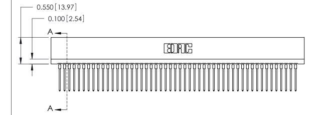
725 Series Ultra-Mate Card Edge Connector - Press Fit
