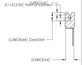
ACAD REFERENCE NO. 746 Series Ultra-Mate Card Edge Connector - Press Fit DRAWN: Part Number: 746-023-553-506 CHECKED: **EDAC INC** THESE DRAWINGS AND SPECIFICATIONS ARE THE PROPERTY OF EDAC INC.,AND TORONTO, ONTARIO SHALL NOT BE REPRODUCED, OR COPIED CANADA OR USED AS THE BASIS FOR THE
