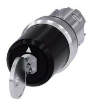
key-operated switch Siemens, 22 mm, round, metal, shiny, lock number SSG10, with 2 keys, 3 switch positions I-O<II, left latching, momentary contact type on the right, actuating angle 2x45°, 10:30h/12h/13:30h, key removal I, with laser labeling, upper case and lower case, always upper case at the beginning of the word
